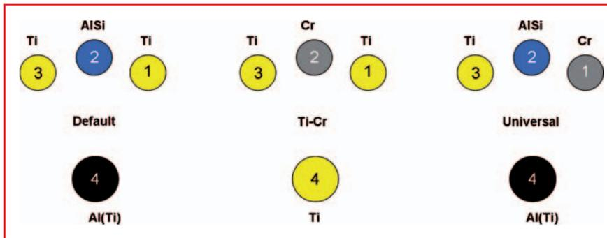
Fig. 3. Three most important cathode configurations of the π313
