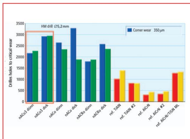
Fig. 5. Triple coatings offer a high capability with minimal variation
