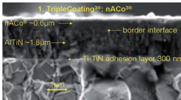
With the aid of the freely programmable stoichiometry, we developed new ›Triple-Coatings‹ (Fig. 4).
